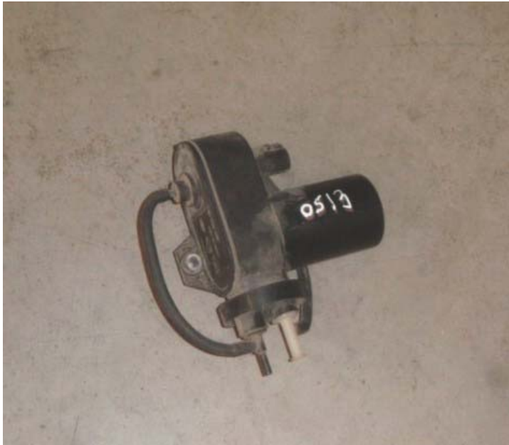
FAILED VACUUM PUMP (1,220 TEST MILES)
