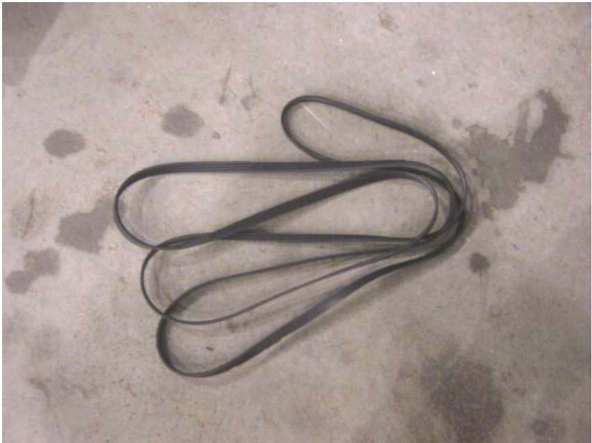
TORN ENGINE ACCESSORY BELT (2,645 TEST MILES)
