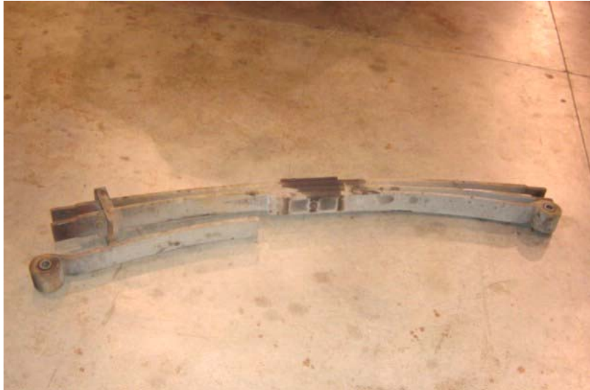
BROKEN TOP LEAF ON THE LEFT REAR SPRING BEAM (3,795 TEST MILES)
