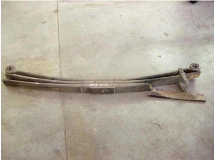
BROKEN RIGHT REAR LEAF SPRING (3,752 TEST MILES)
