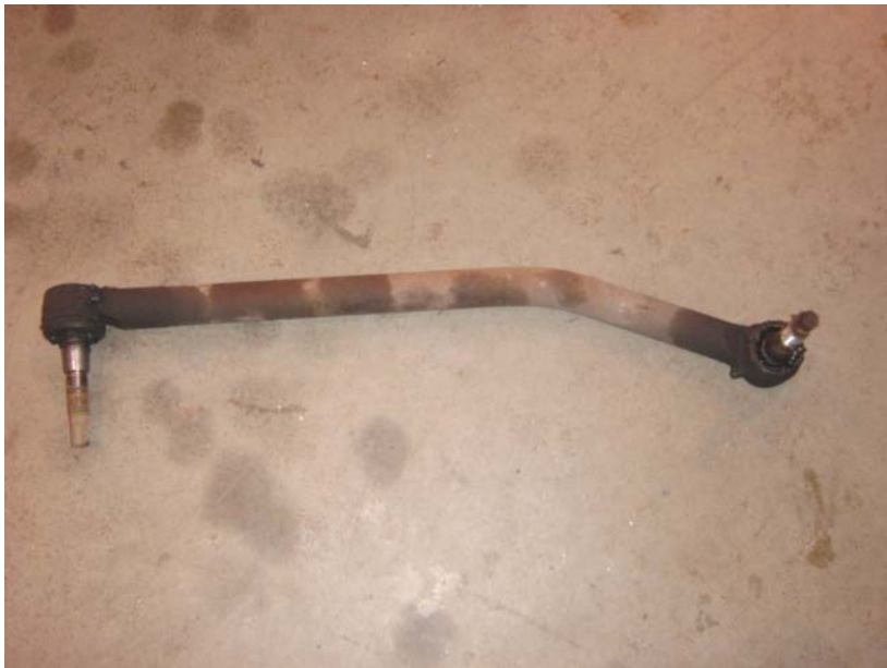
WORN STEERING LINK (9,774 TEST MILES)
