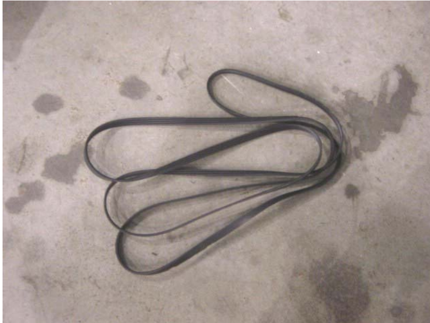
TORN ENGINE ACCESSORY BELT (2,645 TEST MILES)
