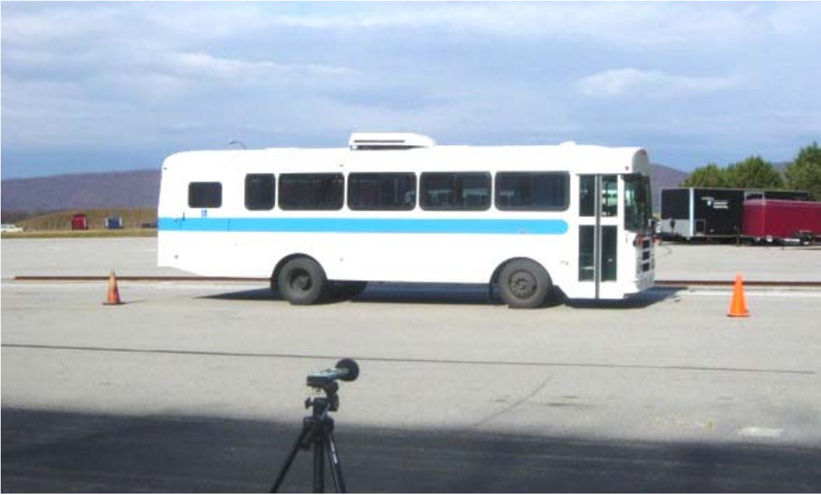
TEST BUS UNDERGOING EXTERIOR NOISE TESTING
