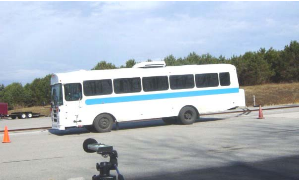
TEST BUS UNDERGOING EXTERIOR NOISE TESTING
