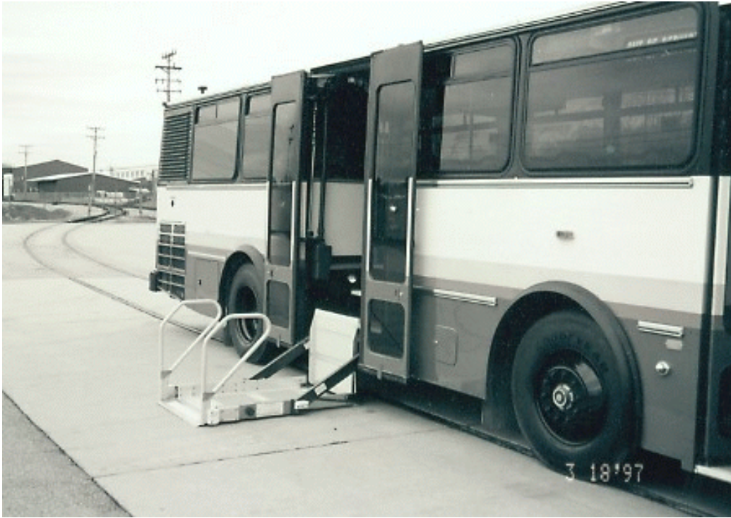
DIAMOND COACH MODEL TC 18 FD EQUIPPED WITH A BRAUN MODEL LZ 11V67 ARS WHEELCHAIR LIFT
