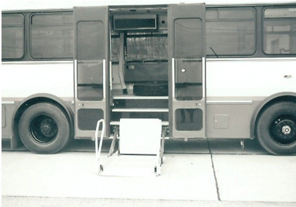
DIAMOND COACH MODEL TC 18 FD EQUIPPED WITH A BRAUN MODEL LZ 11V67 ARS WHEELCHAIR LIFT
