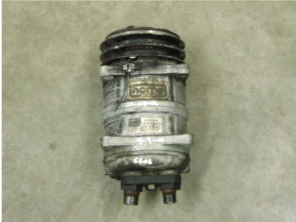
FAILED A/C COMPRESSOR CLUTCH (6,217 TEST MILES)
