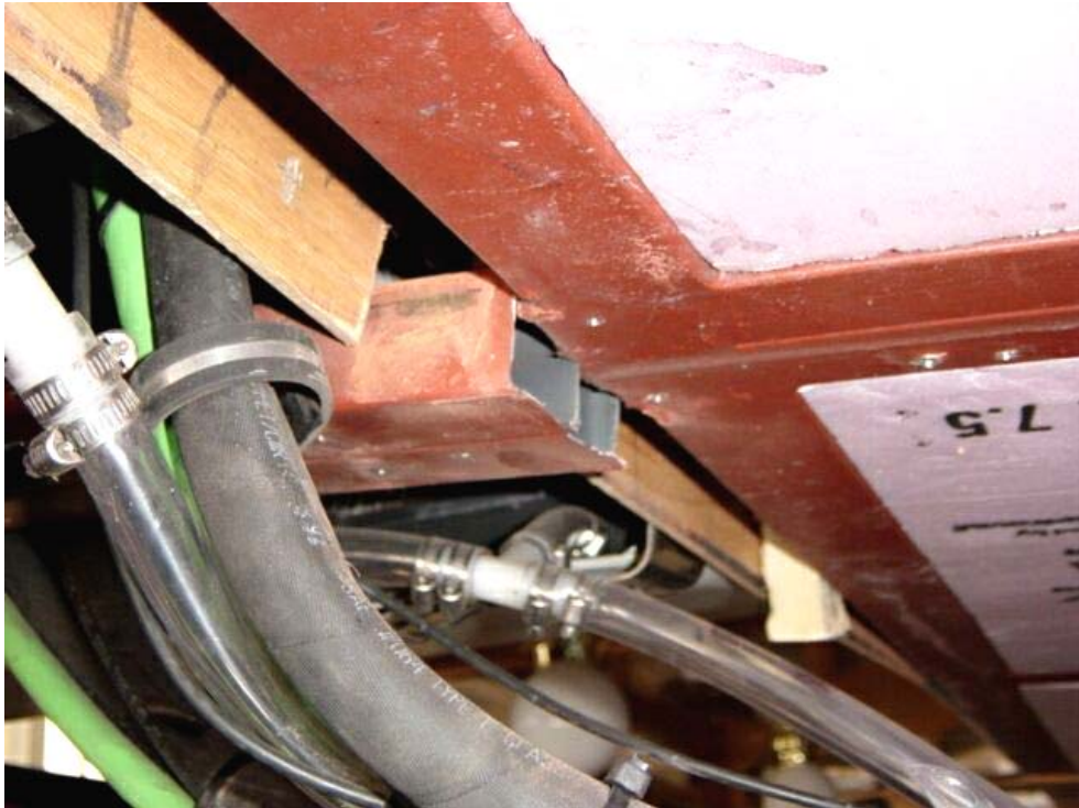
CRACKED ROOF FRAME AROUND THE A/C UNIT (5,927 TEST MILES)
