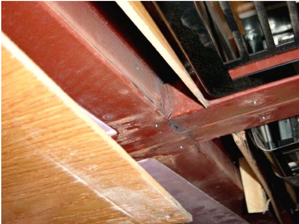
CRACKED ROOF FRAME AROUND THE A/C UNIT (5,927 TEST MILES)
