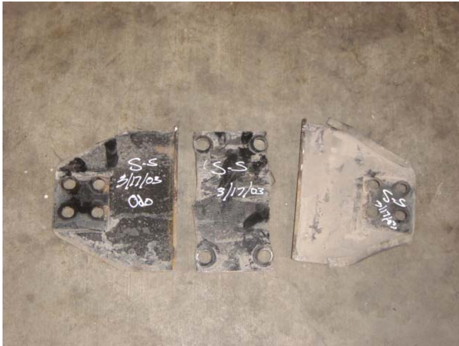
BROKEN REAR SPRING HANGER CROSS MEMBER END BRACKETS (4,267 TEST MILES)
