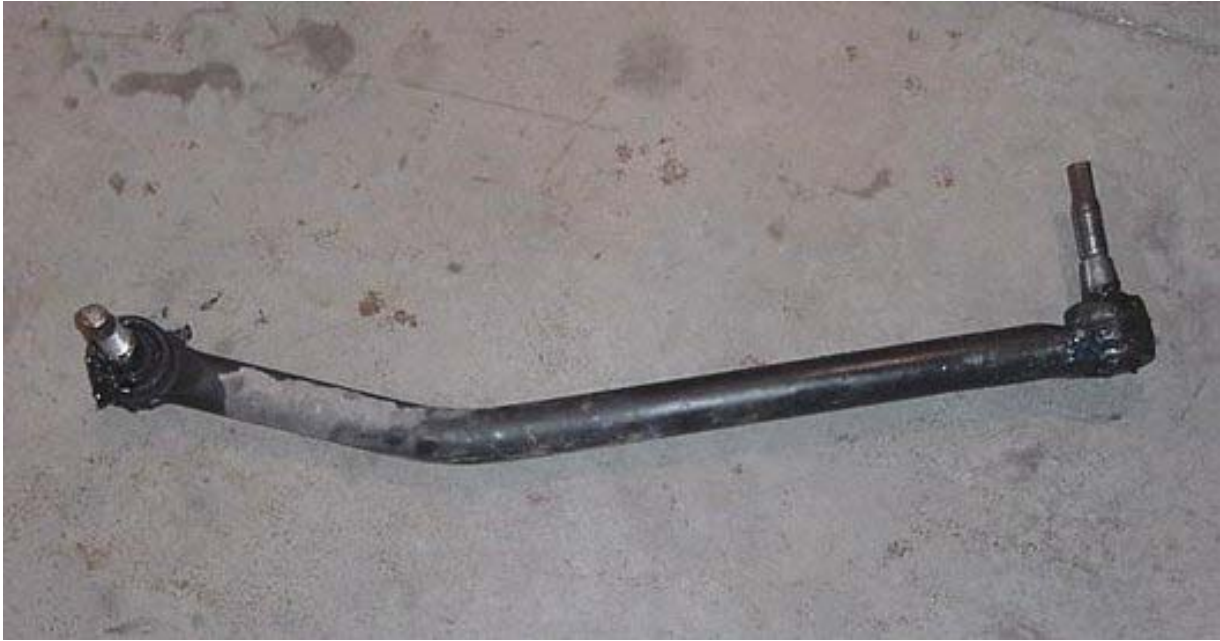
WORN STEERING DRAG LINK (7,849 TEST MILES)
