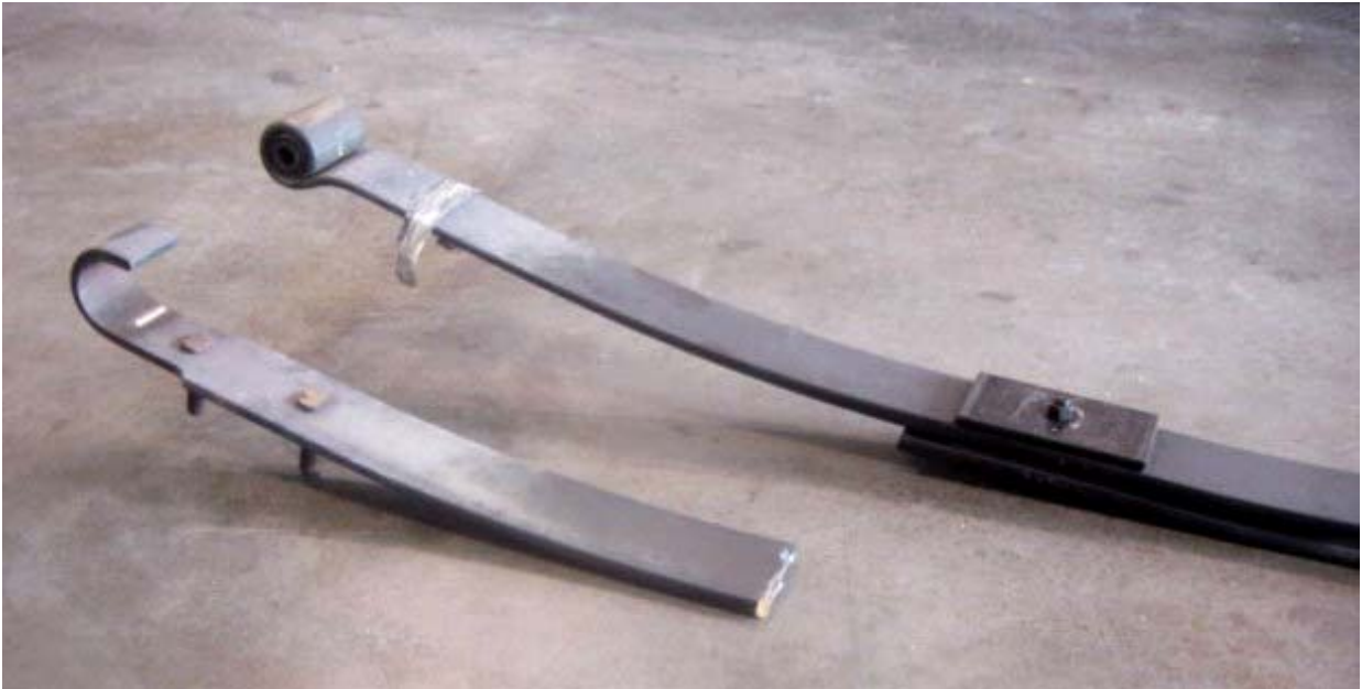
BROKEN LOWER SPRING PLY-- LEFT FRONT SPRING BEAM (1,762 TEST MILES)
