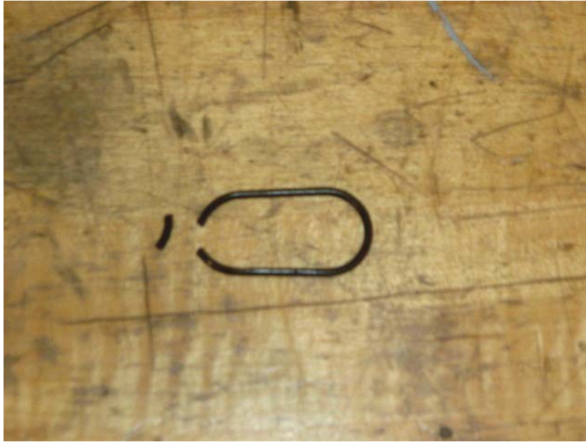
FAILED BRAKE BOOSTER PUMP O-RING (1,288 TEST MILES)
