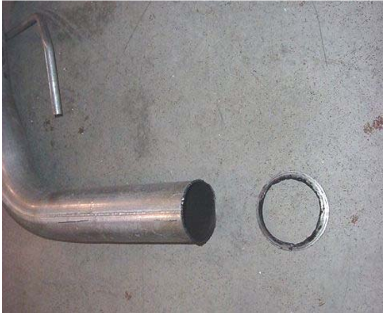
BROKEN FLANGE ON EXHAUST DROP PIPE (5,064 TEST MILES)
