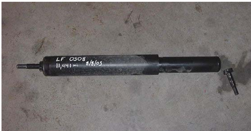
FAILED LEFT FRONT SHOCK (10,436 TEST MILES)
