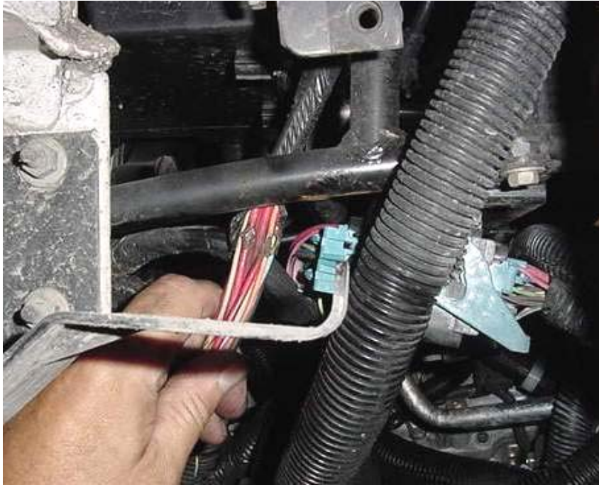
A/C WIRING HARNESS CHAFFING ON THE RADIATOR SUPPORT (7,849 TEST MILES)
